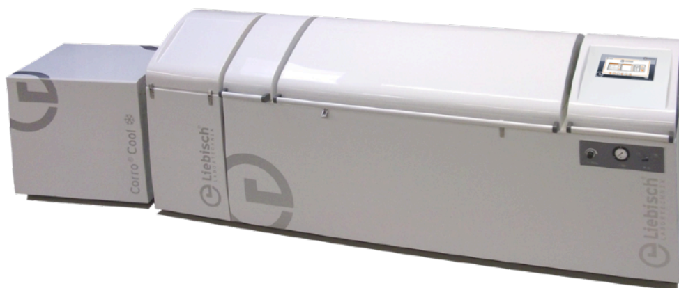
Obr. 11: komora SKBWFCF 1000ATR CORROFROST pro test VDA 233-102
